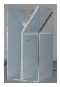
Figure. 3.6 View of the rain gauge to calibrate rainfall intensity
