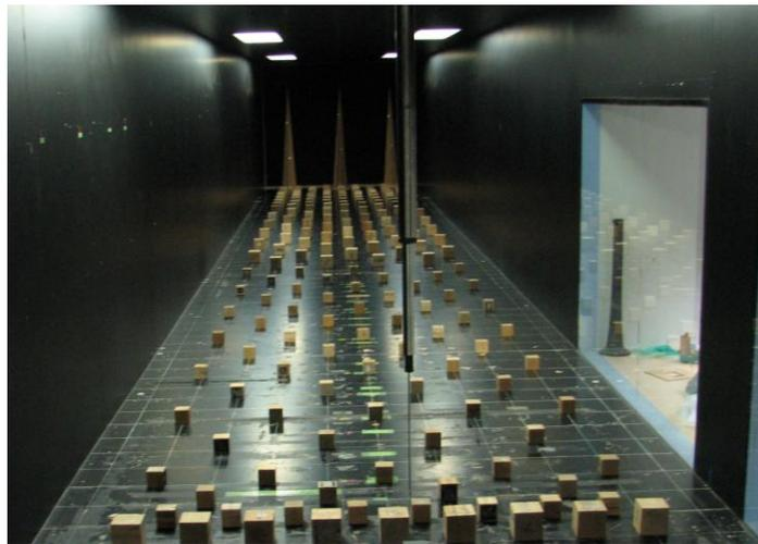
Figure 2.1 Roughness arrangement for Urban flow condition
