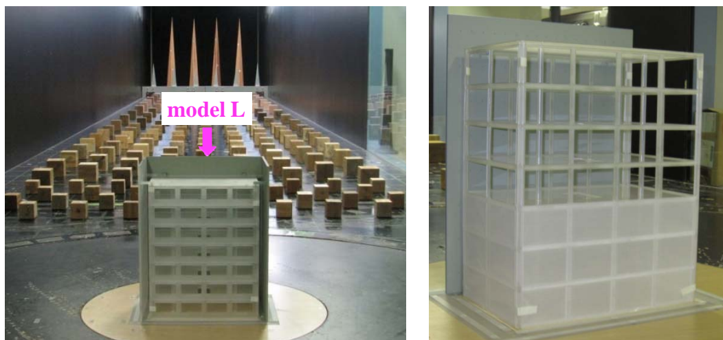
(a) Geometry UL, building opening ratio 40%
