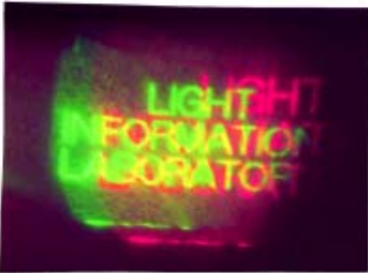
(a) Reconstructed & modified image of OFTH using blue dichroic mirror and He-Cd laser
