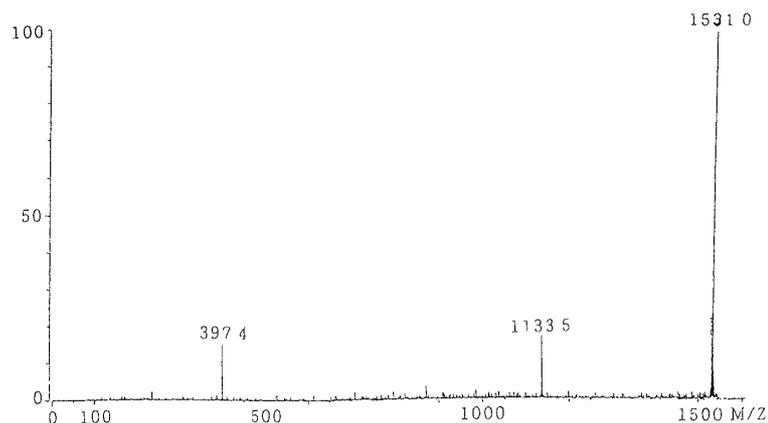
**Fig. 1 Detection of the inclusion complexed ion by FAB-MS spectrometry**
