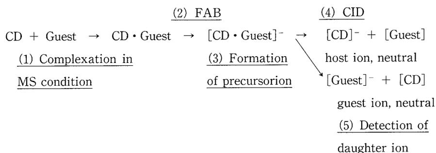
**Scheme 1** The processes (1)~(5) of linked scan FAB-MS to observe the relative ratio of the ionic peak strength, R, as a parameter of complex stability
