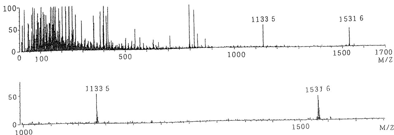
**Fig. 2 Detection of the precursor ion peak and daughter ion peak by linked scan-FAB-MS spectrometry**
