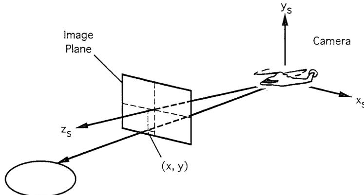
Fig. 2 Image geometry in the camera coordinate system
