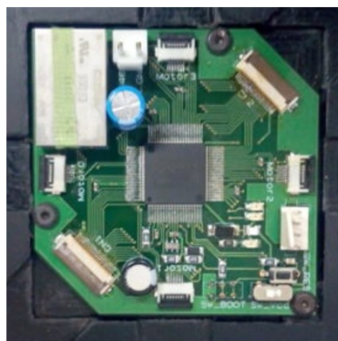
Fig. 2.14: Custom-made control unit
