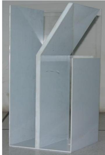
Figure. 3.6 View of the rain gauge to calibrate rainfall intensity
