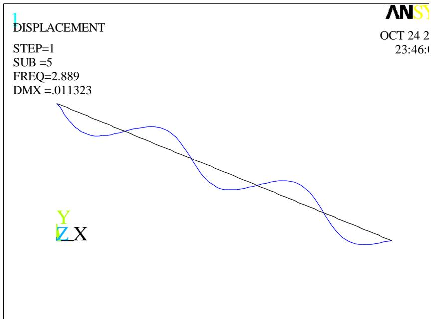
Figure 5.14 3<sup>rd</sup> Symmetric mode of the stay cable
