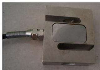
Figure 3.7 S-type Load cell
